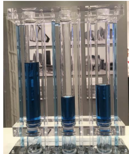
Picture 2: This model compared the flow rates of a typical plain dutch weave with Porometric mesh and optimized dutch weaves (from left to right).
